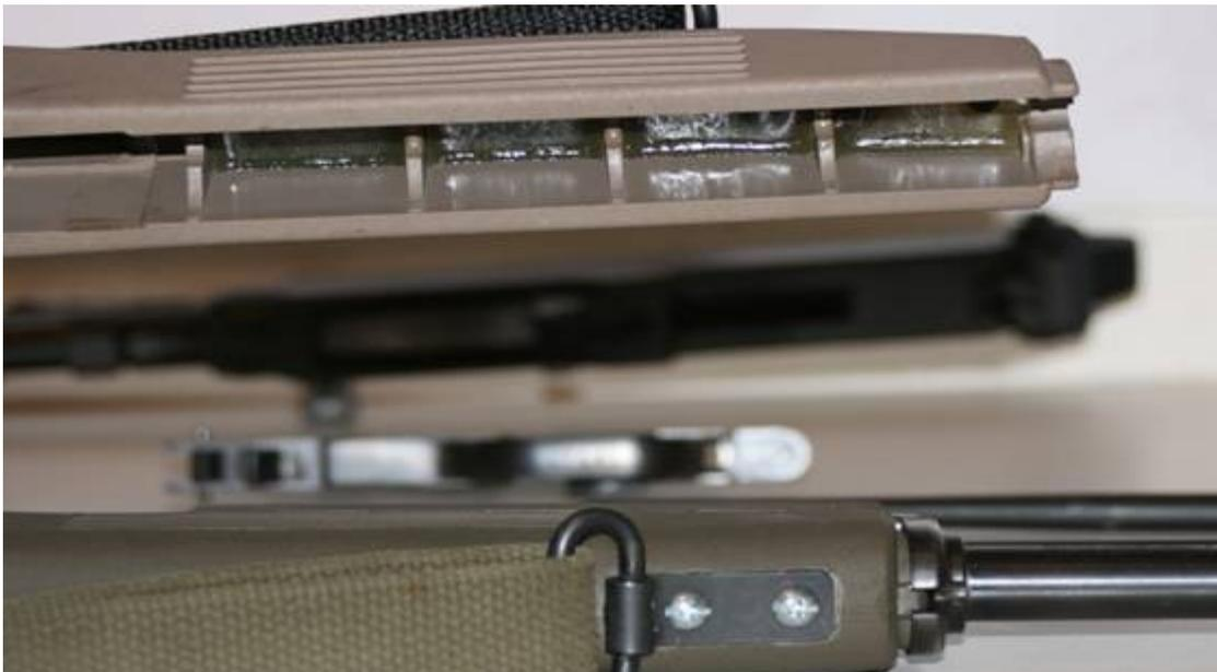
When the compound has set, mark and drill the necessary holes for your swivel type. If using M-14 type swivels, holes may be through drilled and swivel attached with machine screws and nuts.
