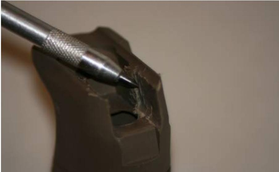
Remove material equally from both sides.
