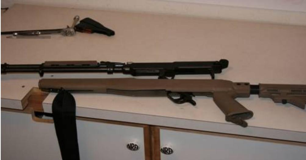
**Top:** Slide trigger group through stock and align front pins in lug. Make sure that disconnect bar aligns properly in upper receiver.
