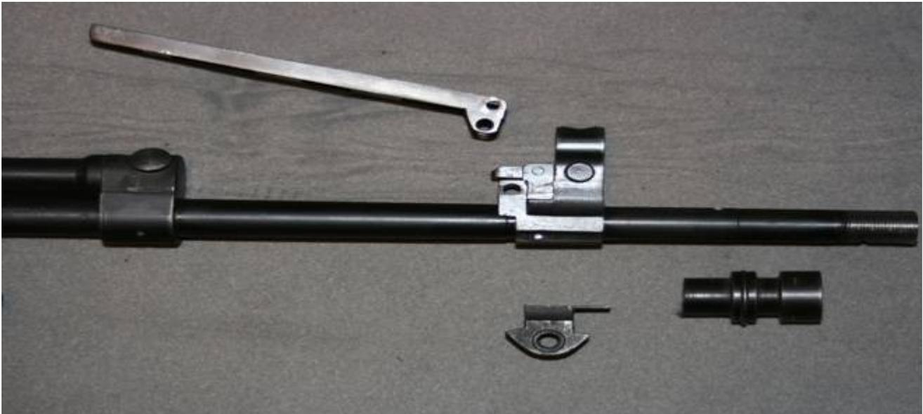
Note pin relief cuts in barrel. This example still has the flip up night sight.
