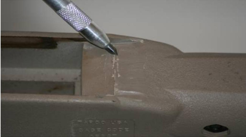
3-Front sling swivel. We chose to use the M-14 front sling swivel, other types may be used if desired. All swivels will require the following stock modification, using fiberglass resin, epoxy, or similar compound (see photo). Fill the bottom inside of the forearm to a depth of at least ½” in the area where the swivel will be mounted.
