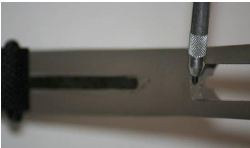
8-Break sharp corners and edges. Using sandpaper or small file deburr mold marks, mag well edges, pistol grip, etc. for comfort and looks.
